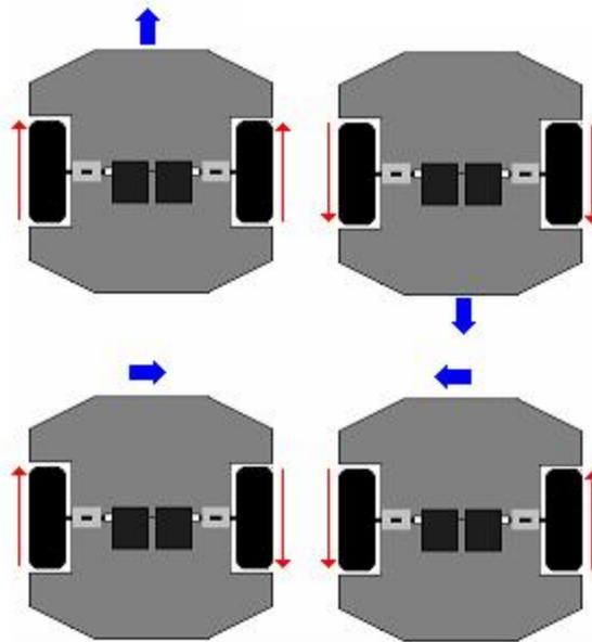
The differential drive is perhaps the most used drive when it comes to the field of robotics.
